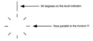
You will probably need a small flashlight to alternately view the level indicator and then look through the eyepiece until everything is lined up. When I started using this technique, I noticed a dramatic increase in the accuracy of my polar alignments for CCD imaging without going through the lengthy process of dec. drift alignments, etc. This technique is very good if you are mobile most of the time, etc. Hope it helps you out. Good luck.
