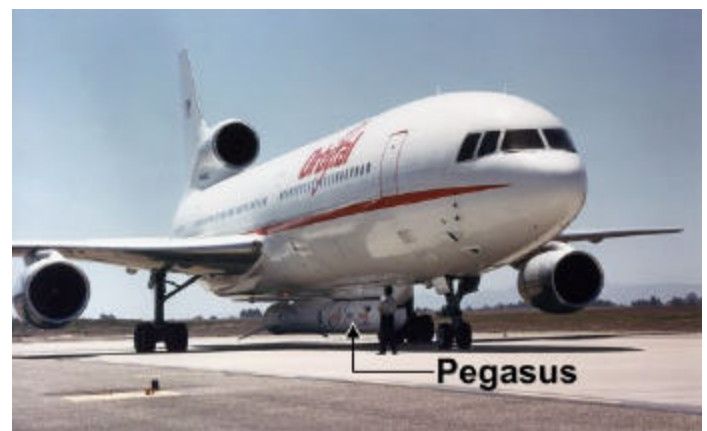
L-1011 "Stargazer" takes off to carry Pegasus rocket on the first 39,000 feet of its climb to deliver a spacecraft to orbit.
