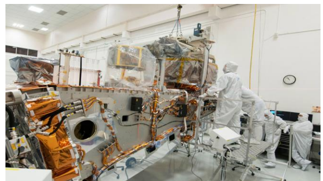
Caption: Ball and Raytheon technicians integrate the VIIRS Optical and Electrical Modules onto the JPSS-1 spacecraft in 2015. The spacecraft will be ready for launch later this year. Image Credit: Ball Aerospace & Technologies Corp.
